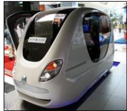
Picture 12. PRT Podcar fits 4-6 people, goes faster than a bus and functions without a driver.
